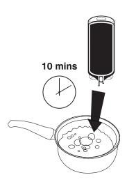
squeeze metal disk inside to activate heat for 10 mins in hot water to charge for re-use
